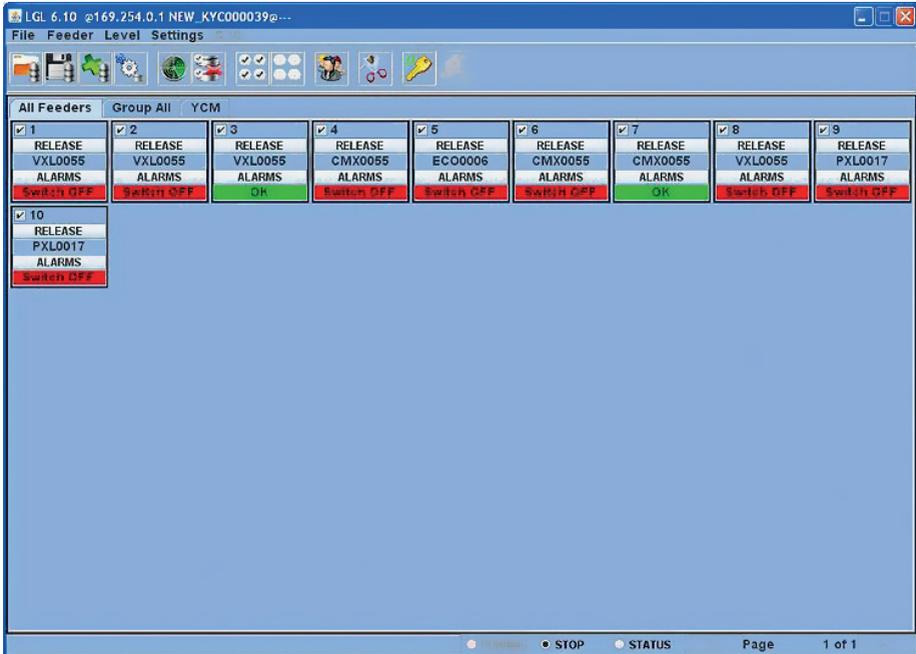
STATUS TAB located at the bottom of the screen: alarm monitoring in continuous mode. This feature is necessary if the computer is far from the machine, in order to be able to have information on possible alarms without being at the machine. In case an alarm takes place while the machine is running and the STATUS tab is selected, the feeder will stop the machine and a big writing will come out on the display as in the following picture:
