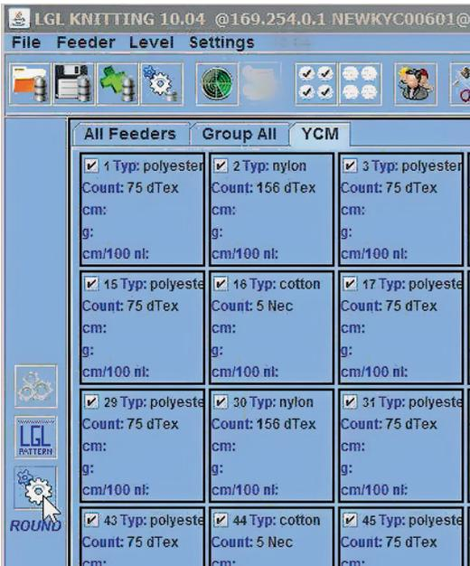
The system calculates the yarn consumption in a pattern taking its length in terms of number of machine revolution.
