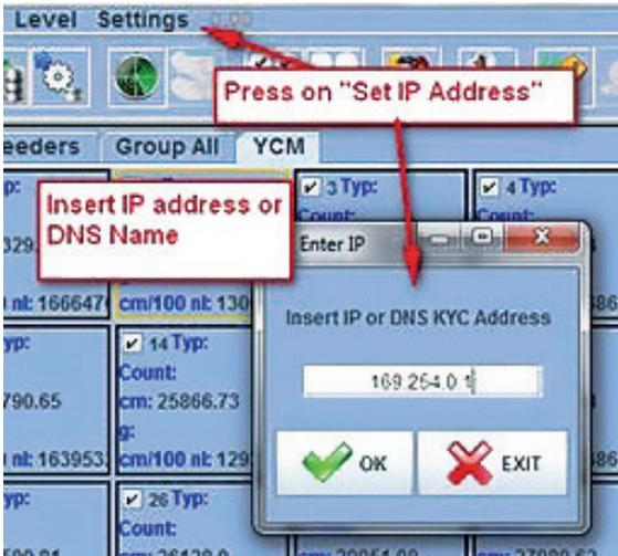
B. Press **Settings – Set IP address**. Insert the address of the KYC (169.254.0.1 in the example of the picture).
